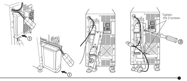
6. Securely connect the upper and lower connectors. ① Secure the connector to the plate cover. ②
